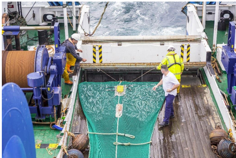
Figure 6. Fishing net on-board after a fishing haul, with the WiSens CTD sensor attached (within the orange case), during Pelacus0422 cruise.
