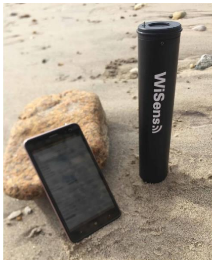
Figure 1. The NKE WiSens sensor can be accessed and configured with any device with Wi-Fi connectivity.
