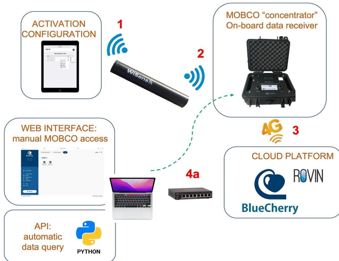
Figure 3. Scheme of the FOS connectivity and data management: 1) activation of the WiSens sensor with a magnetic clip and configuration via Wi-Fi; 2) data transferring to the on-board receiver (MobCo) via Wi-Fi; 3) MobCo connection with the BlueCherry.io service via 4G network; 4) MobCo can be accessed and thus data downloaded in two different ways: i) manually, through BlueCherry.io service, and ii) automatically (as in the experiences presented in this report) by means of an Application Programming Interface (API) (in our case, developed by IEO-CSIC technical staff).
