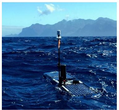
The glider, belonging to Island the Canary Oceanic Platform (PLOCAN), was released on the 16<sup>th</sup> of October and recovered on the 23rd of November 2018. During those 35 days, the surface glider travelled 1539 km collecting meteorological oceanographic and variables, including noise level in the ocean by using
