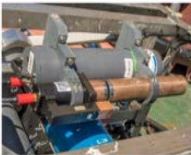
Satlantic SUNA SN 745 nitrate sensor (plastic housing, wrapped in copper tape) with integrated wiper deployed on the sensor frame
