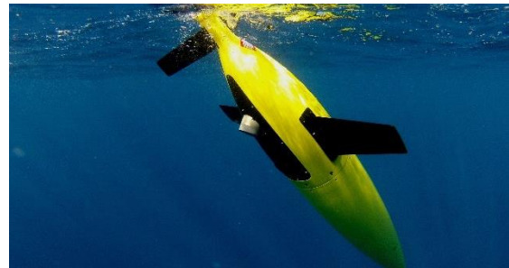
Figure 3 SeaGlider as example of underwater (buoyancy-driven) glider technology
